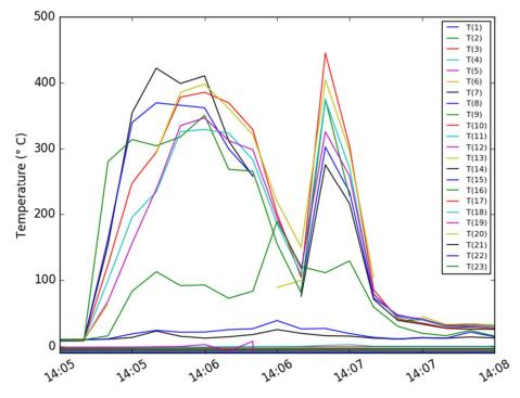
Figure 9. Enlargement to show flame temperature development.
