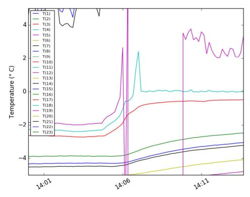
Figure 10. Enlargement to show temperature development in the upper ice layer. T(10) and T(11) are shown in red and cyan, respectively.
