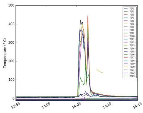
Figure 8. Overview of temperature measurements. T(1) through T(12) are in the ice, cf. Table 1.
