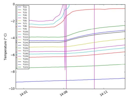
Figure 11. Enlargement to show temperature development in the lower ice layer.
